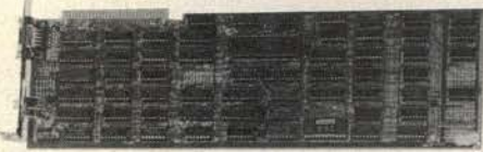
E) COLOR GRAPHICS ADAPTER *Has standard 6845 color graphics controller chip. *Capable of driving R.G.B. monitor, color monitor, black and white monitor, home TV (user-supplied RF modulator) *Test mode 40 column x 25 row color/black and white 80 column x 25 row color/black and white *Graphics mode 320 dot x 200 line color/black and white 640 dot x 200 line black and white Light-Pen interface is available
